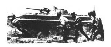
Figure 6-12. Troops in the offensive. Riflemen can attack in their APCs or dismounted. Shown here is the new BMP amphibious armored infantry combat vehicle, which provides armor protection for eight infantrymen, fire support from its 73-mm gun, and anti-tank defense with SAGGER missile launchers.
